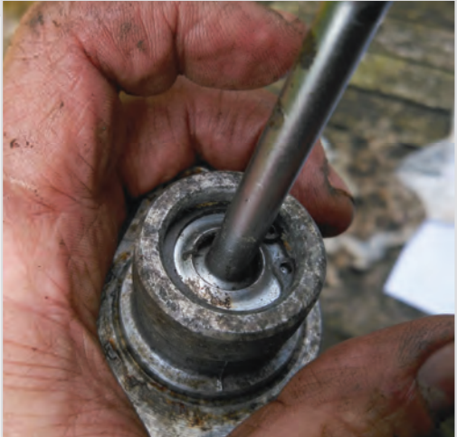
Circlip back in place holding the actuating rod assembly in place.
