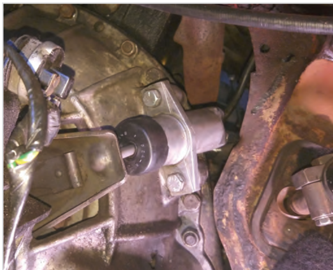
Rebuilt slave cylinder re-fitted
