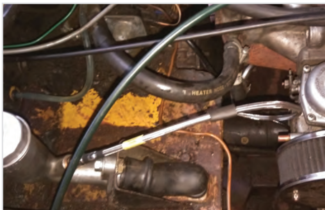
Master Cylinder installed with New Clutch hose
