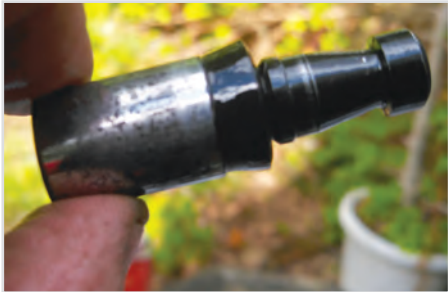
Piston Seal fitted, note the wide lip faces away from the piston.
